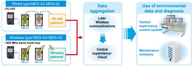
\* A gateway is required separately for remote monitoring.
