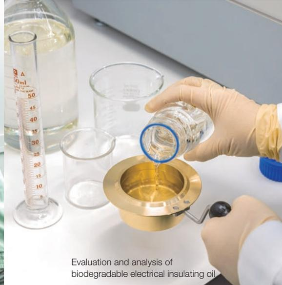
Evaluation and analysis of biodegradable electrical insulating oil
